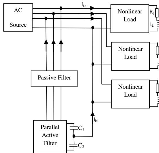
Figure 2. Three phase 4-wire hybrid active power filter with split capacitors.
