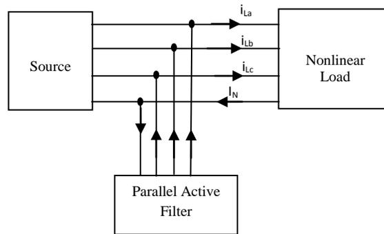
**Figure 1.** Three phase 4-wire shunt active power filter.
